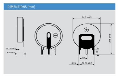
$<sup>^{*}</sup>$  In applications where the battery is exposed to temperatures >60  $^{\circ}$ C, please contact Jauch.
